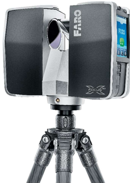
Photo. 1. Laser scanner FARO Focus 3D;
